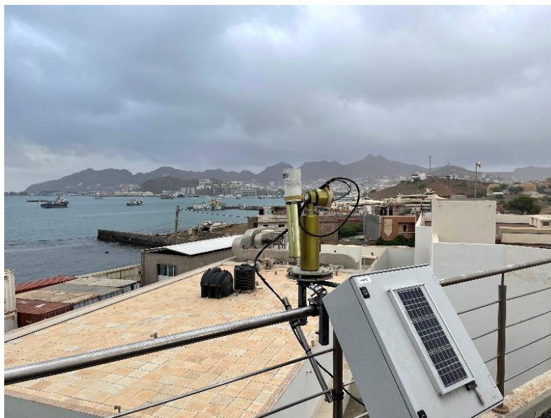
Figure 26: The CE318 photometer from CIMEL on the rooftop of the OSCM, Cape Verde.
