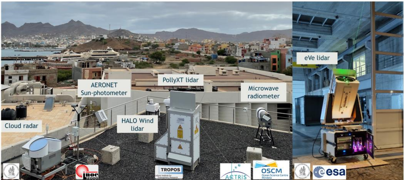
Figure 20: The ACTRIS ground-based instruments installed at the OSCM premises for the ASKOS experiment.
