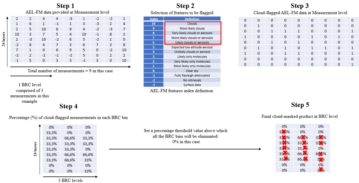
Figure 3.2: A graphical illustration of the cloud-filtering methodology using the AEL-FM feature mask product.
