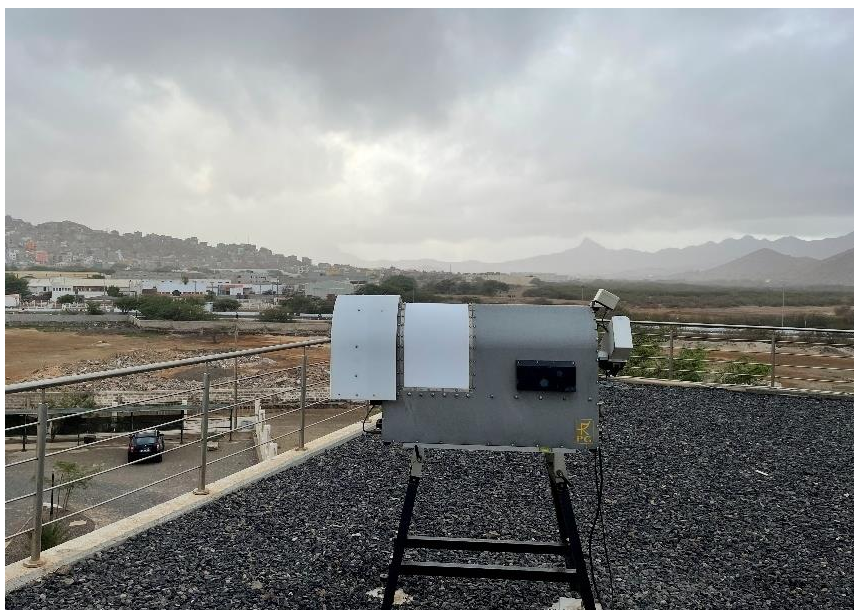
Figure 29: The RPG microwave radiometer installed on the rooftop of the OSCM, Cape Verde.
