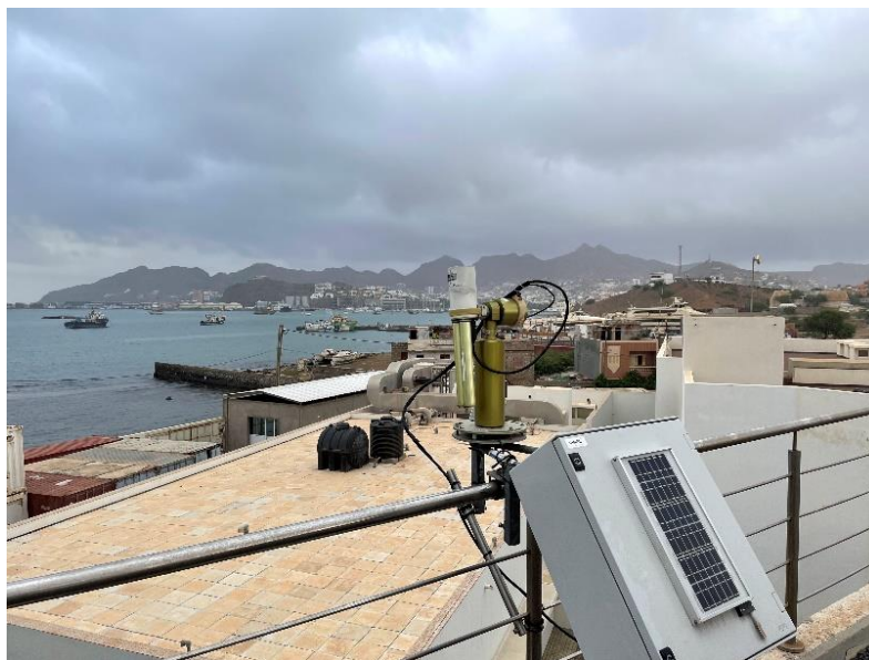
Figure 27: The CE318 photometer from CIMEL on the rooftop of the OSCM, Cape Verde.
