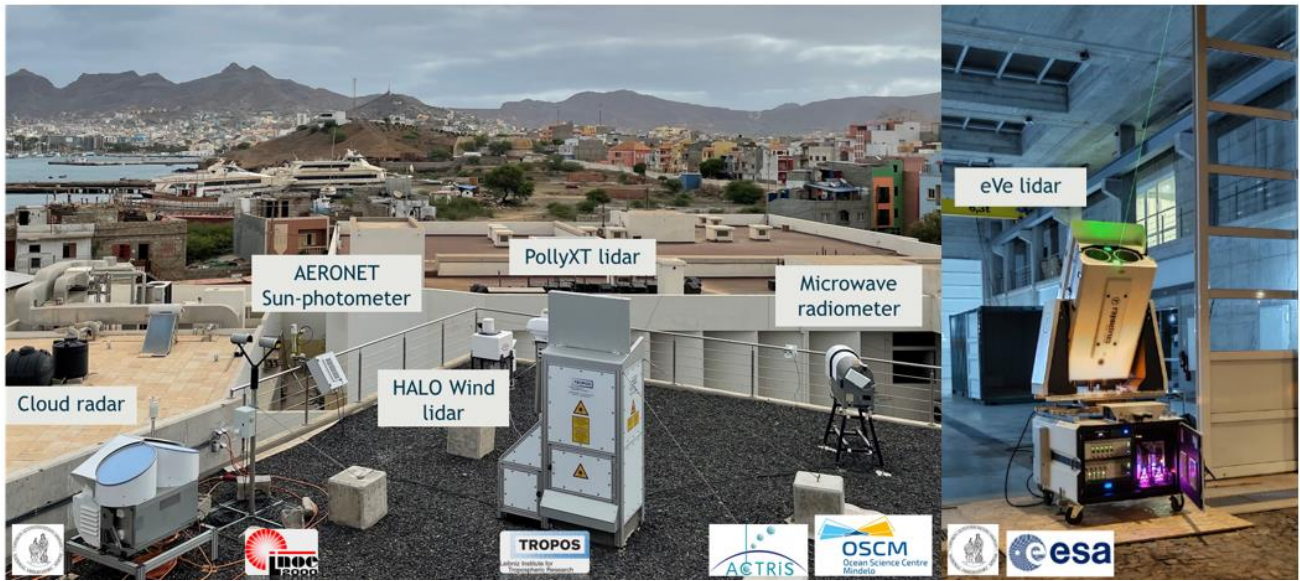
Figure 21: The ACTRIS ground-based instruments installed at the OSCM premises for the ASKOS experiment.
