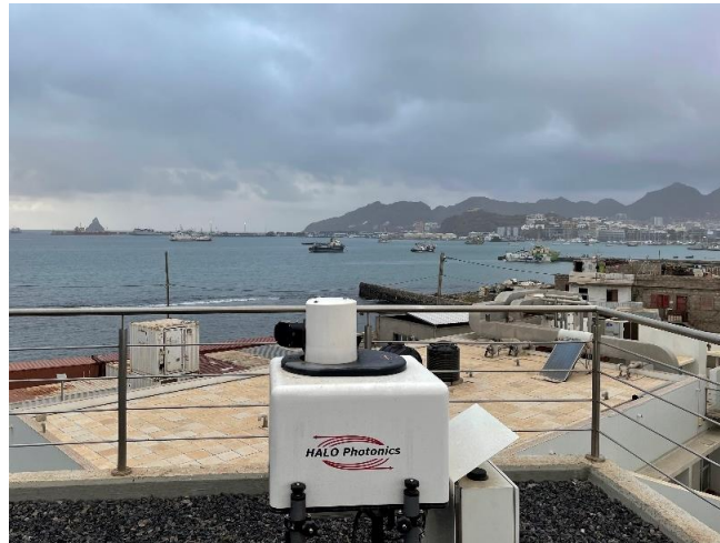
Figure 26: The HALO Streamline-XR Doppler wind lidar on the rooftop of the OSCM, Cape Verde.
