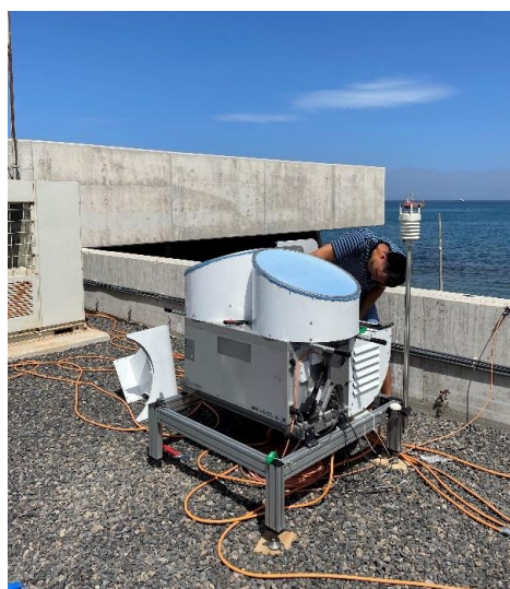
Figure 31: The installation of the 94 GHz FMCW Doppler Cloud Radar on the rooftop of the OSCM, Cape Verde.
